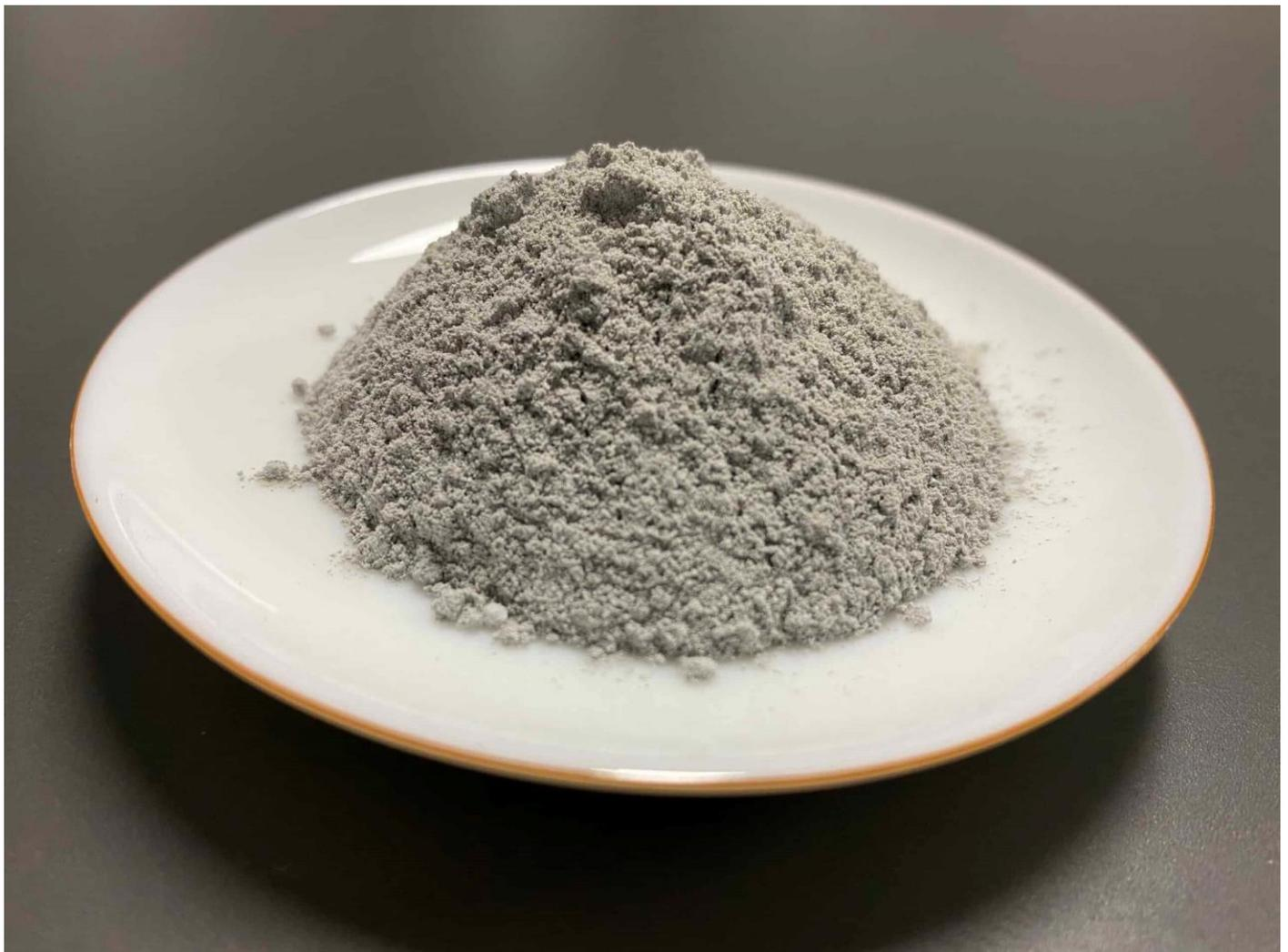
Although there is no clear difference between densified and undensified apart from the density, densified silica fumes still offer some advantages. These advantages include:
